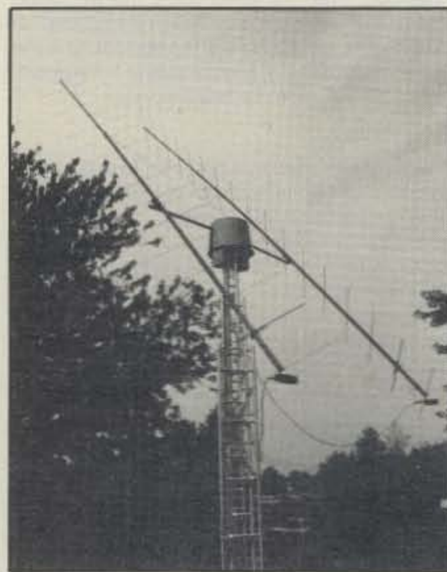
Fig. 1— Complete antenna. Distance between the booms is 6 feet. Note coax falling away from reflector.
