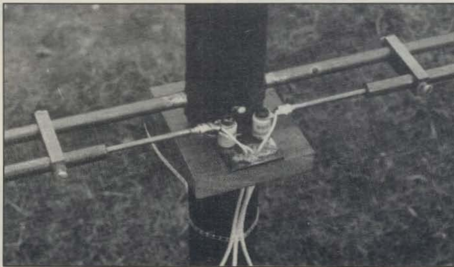
Fig. 2— T-match. Coax is soldered to ring lug which holds the center rod.
